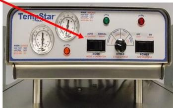
The Delime Switch! Lime build-up is the result of hard water running through your machine. Commercial dish machines are absolute workhorses, and yet many operators hardly ever use the delime cycle which is built into their equipment. WTF?
