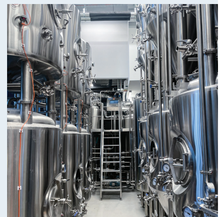
7bbl direct fire system with stacked tanks
